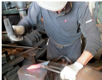
The first step in making a sickle: wedge steel in between the iron, melt it in a forge that is of 1000 degrees Celsius, and hit it with a hammer.
