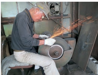
Finishing touches are made to the raw blade with a grinder before quenching it in water.
